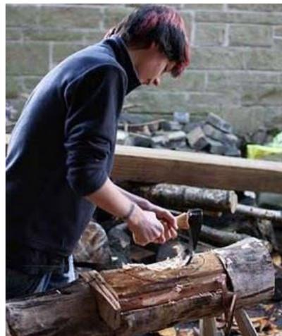
A good adze is a remarkable tool and quite quickly it is possible to be remarkably accurate. The adze is followed by a gouge for smoothing and refining the form.
