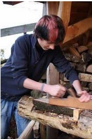
With the blank turned and wedged he starts hollowing with an adze.
