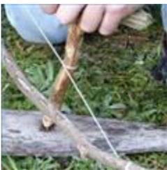
Lean down over your left knee and press down slightly on the handhold with your left hand. Move your right arm back and forth in a sawing motion, causing the spindle to spin back and forth.
