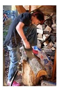
Axing the base of the bowl flat and removing all the pith.
