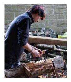
A good adze is a remarkable tool and quite quickly it is possible to be remarkably accurate. The adze is followed by a gouge for smoothing and refining the form.
