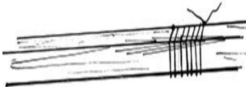
If the fibers start to split off, quickly wrap that place with string, keeping the fibers intact. Continue bending gently.
