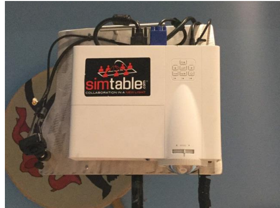
22) Level the projector with slight adjustments. This can be challenging we have used packing tape from the projector base to the tripod to assist with leveling.
