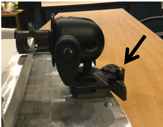
19) Tripod head connected to projector base making sure the latch locks in place.
