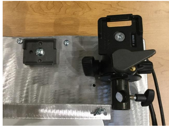
18) Tripod head to connect to projector base
